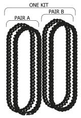
NOTE: DIAMOND CHAIN WILL SUPPLY THE FULL KIT OF COMPONENTS THAT WILL PROVIDE FOUR CHAINS FOR ONE COMPLETE INJECTOR UNIT AS SHOWN ABOVE. THE CHAINS WILL BE SUPPLIED LOOSE, TO BE ASSEMBLED BY THE USER.
