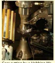
Gear cutting by a Hobbing Machine
