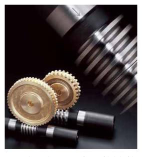
An arrow marking on the outer circumference of the hub of the KHK duplex worm indicates the direction of assembly as well as acts as a guide for the backlash adjustment.
